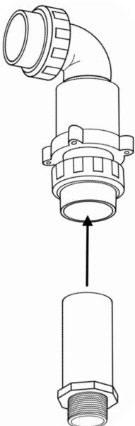
Use a small piece of sandpaper to smooth out the cut end of the discharge pipe. Clean the 2" socket fitting on the bottom of the check valve and the cut end of the discharge pipe with PVC cleaner/primer. Apply PVC glue and insert the discharge pipe into the 2" socket fitting. Hold the discharge pipe firmly in place for a few seconds, giving the glue time to set.
