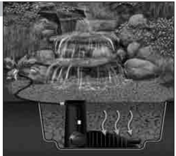
Fig. 2 & 3 Ideal placement for MicroFalls®, MicroSkim® and plumbing.
