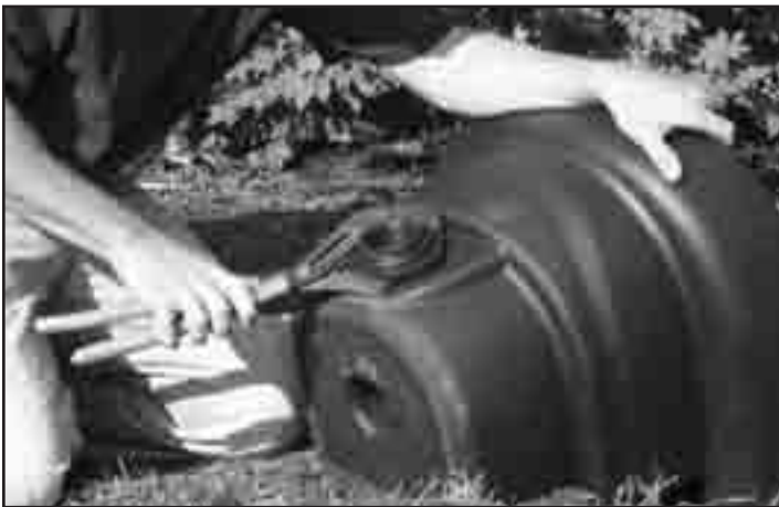
Fig. 4 Attach bulkhead fitting.
