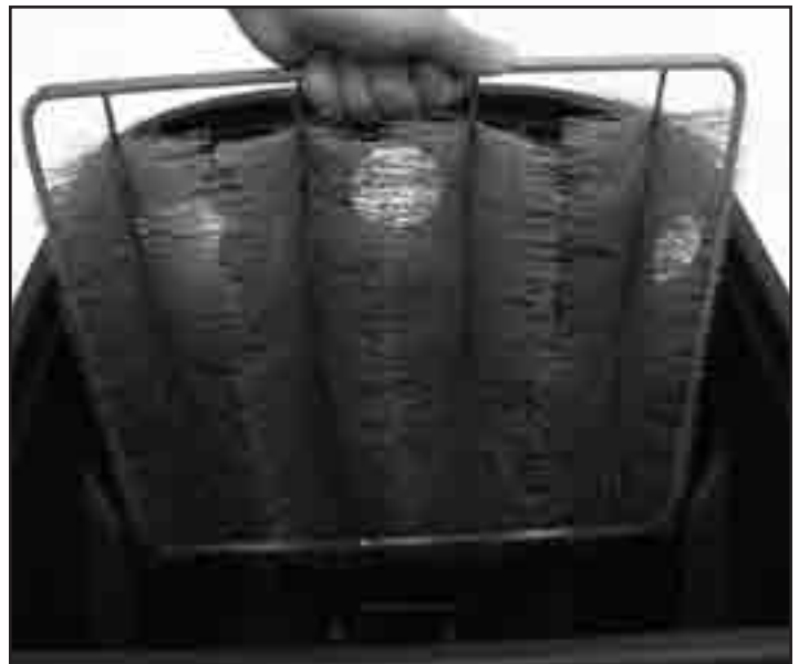
Fig. 44 Filter brush cartridge inside the skimmer
