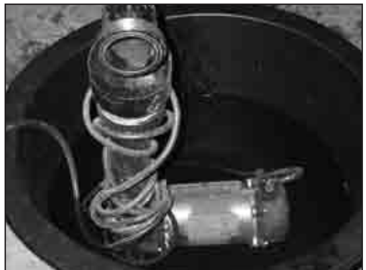
Fig. 51 Store the pump in a frost-free location, ideally submerged in a bucket of water.
